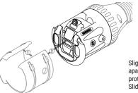
Slightly push the protective cover apart so that it can slip over the protruding screw head (1). Slide the protective cover onto the camera from the front (2).
