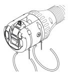
Secure the retaining rings by placing them with the opening against the recess and then by sliding them over the shell with firm pressure.
