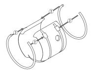
Slide the retaining rings over the protective cover and insert them into the provided recesses of the protective cover (2).
